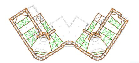
W-shaped building with a façade height of 18.2 m, which means 146 ml of façade and 2657 m2 of wall surface to be preserved.
