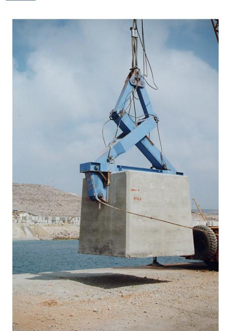
Friction clamp for the movement of 40 tonne blocks. Port of Carboneras.
